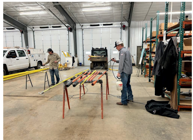
Brent and Brock testing hot sticks.
