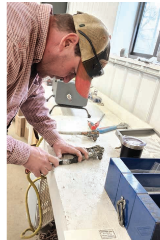
Lineman Brock Fischer tests hot sticks. Insulated hand tools designed to protect crews when energizing or de-energizing power line.
