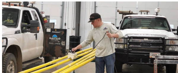
Lineman Brock Fischer tests hot sticks. Insulated hand tools designed to protect crews when energizing or de-energizing power line.
